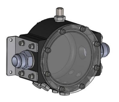
The air bleed/return manifold allows connection of multiple return lines to the system reservoir, while providing a natural high point for air within the system to naturally accumulate when oil flow is static. A clear front screen allows any trapped air pocket to be easily seen and vented.
